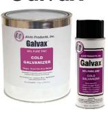
Zinc-rich cold galvanizer. Protects metal surfaces. The 95% pure zinc cold galvanizing compound electro-chemically bonds with metals to stop rust creepage and corrosion. Sprays or brushes on cold. Heals itself when scratched. A coating of Galvax is comparable to hot-dip galvanizing for metal protection. Cures damaged hot-dip coatings and repairs damaged galvanized surfaces. Used for
